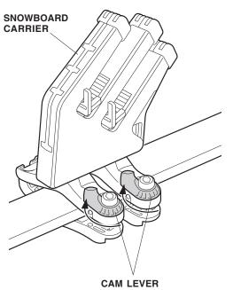
CAM LEVER Return to the original location. 10. To prevent theft, install the screws in the holes in the top clamps.
